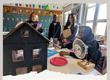
BEFORE WINTER BREAK, SENIORS SPENT A FEW WEEKS IN Engineering Physics, designing and constructing model Passive Houses. A passive house is intentionally designed to Utilize the passive heat from the sun as its main energy Source and thus doesn't need a furnace.. Making it Incredibly energy efficient! Students tested their models For both a temperature increase and thermal maintenance.
